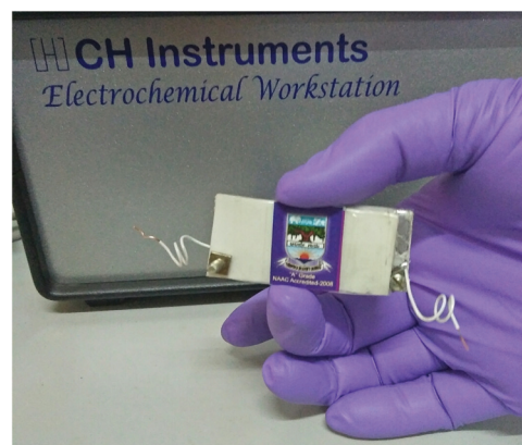
Fig. 3 The photo image of the fabricated sandwich-type device.
